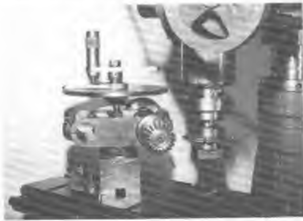
Fig. 82 The bevel wheel shown in the last photograph after the first pass of the cutter through all the teeth.
